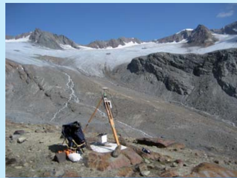
Picture 2: A relative gravimeter LCR-G observing at a reference station on solid rock.
