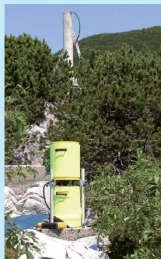
Picture 1: The mobile absolute gravimeter A10 owned by the BKG during measurement close to the GPS pillar (in the background) of the GAIN station at mount Wartsteinkopf in 2005.
